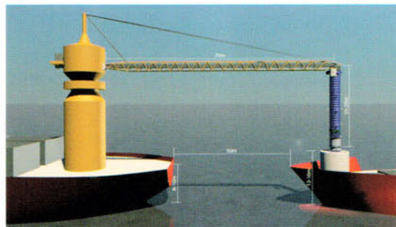
Cargo handling system FPSO - hydrate pellet carrier.
